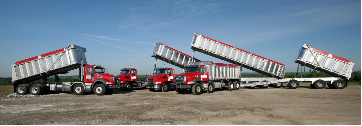
James Dick Gravel Fleet Trucks Types. Left to Right: Tri-Axle Straight Truck, Tri-Axle Tractor Trailer, Quad-Axle Tractor Trailer, Tri-Axle Pony Pup Combination.
