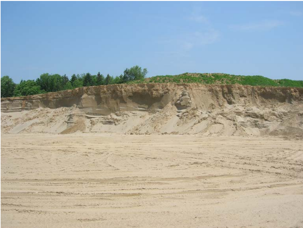
Figure 2. Vertical sand face (+/- 8m) during active extraction.
