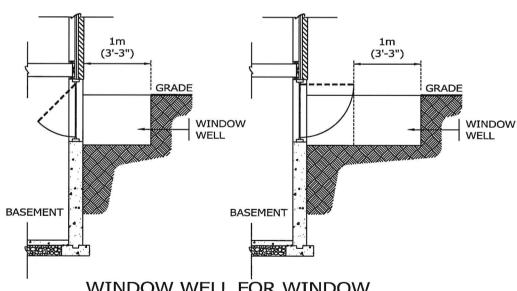
WINDOW WELL FOR WINDOW PROVIDING ADDITIONAL MEANS **OF ESCAPE**
