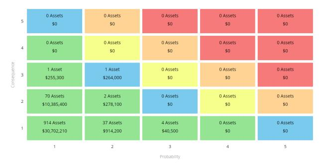
This is a high-level model developed for the purposes of this AMP and Township staff should review and adjust the risk model to reflect an evolving understanding of both the probability and consequences of asset failure.
