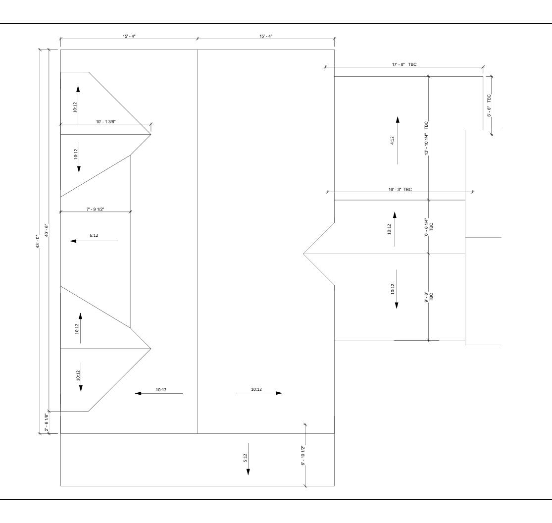
ALL EXISTING DIMENSIONS TO BE CONFIRMED BY THE CONTRACTOR PRIOR TO CONSTRUCTION & PRODUCTION OF PREFABRICATED PRODUCTS SUCH AS PRE-ENGINEERED WOOD TRUSSES. THE DESIGNER MUST BE NOTIFIED OF ANY MAJOR DISCREPANCIES BEFORE WORK COMMENCES
